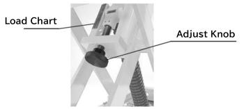
Load capacity increases when turning Adjust Knob counterclockwise, and decreases when turning clockwise. Load can be adjusted to any capacity within loading diagram range.
